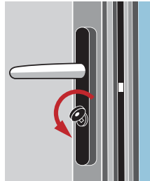
Fig 24. Step 3 – Some front door applications require a turn of the key to retract the latch bolt from outside. Turn the key away from the lock edge to retract the latch bolt.
